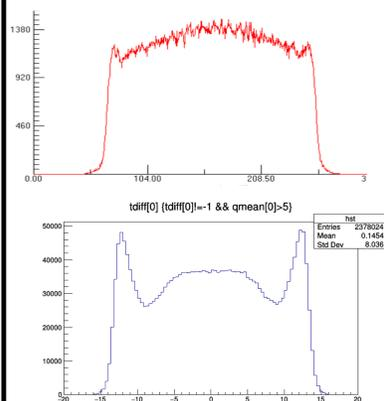
Top: An analog graph of cosmic muon position data. Light attenuation reduces counts near the ends of the bar as lower energy events drop below threshold since light has further to travel. Note a gentle slope.
