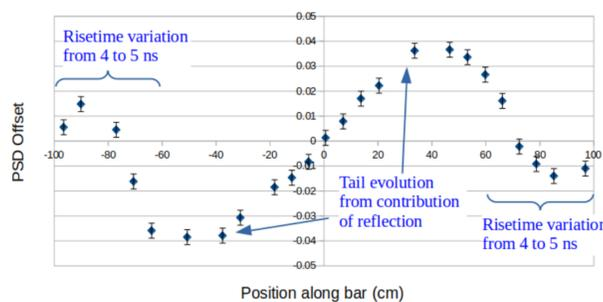
Graph to the right shows near and far waveforms. Rise time varied from 4ns (near) to 5ns (far). A plot showing the evolution of the waveform shape via its PSD spectrum. The nonlinearity is evident in this plot for the outer 40cm of each end.
