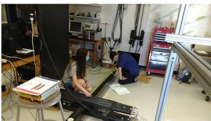
We placed half-sized scintillator bars above and below the MoNA bar, then found triple coincidences from cosmic muons across the three detectors to determine precisely where a muon hit. In total, we took muon data at 30 positions across the bar's length, in 6.5cm increments. Measuring the physical position allowed us to evaluate our **mapping from time difference (channels) to calculated position**.
